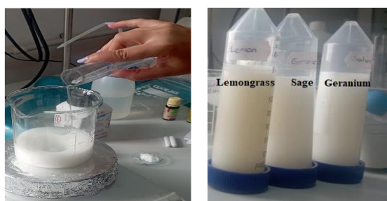
Figure 3. a) Photographic image of sample 1 – multiple emulsion based on Tween 20/Tween 80/Lauryl Glucoside; b) Photographic images of: sample 2 – multiple emulsion based on Tween 20/Tween 80/Lauryl Glucoside and geranium extract; sample 3 – multiple emulsion based on Tween 20/Tween 80/Lauryl Glucoside and lemongrass extract; sample 4 – multiple emulsion based on Tween 20/Tween 80/Lauryl Glucoside and sage extract
