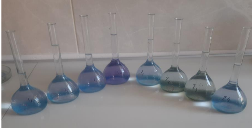
Figure 2. Flasks with analytical solutions prepared for use on the spectrophotometer (first four flasks on the left – after 0.5 h of bating, last four flasks on the right – after 1.0 h of bating)
