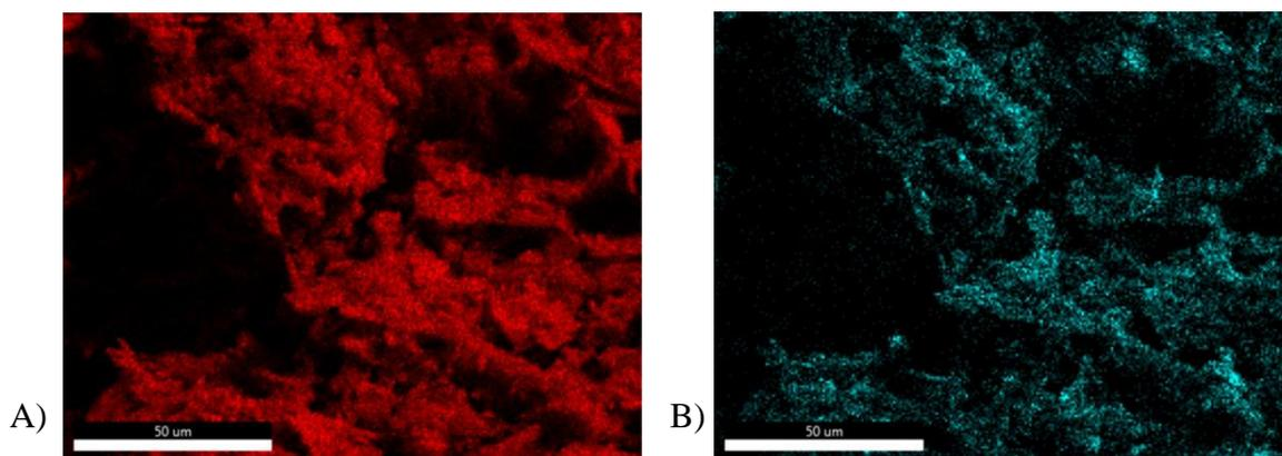
Figure 8. X-EDS maps for carbon (A) and oxygen (B)
