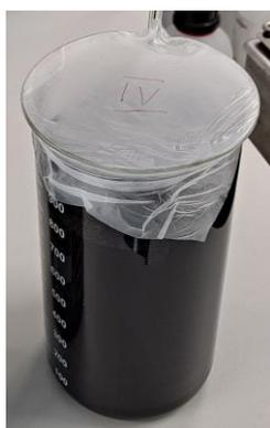
Figure 2. The prepared conductive carbonic paste
