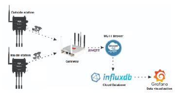
Figure 2. Architecture of the system
