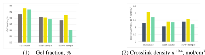
Figure 4. Gel fraction and crosslink density of samples for: normal state (dark gray), after the thermophilic incubation period of 42 days (yellow), and after the thermophilic and mesophilic incubation period 84 days (green)
