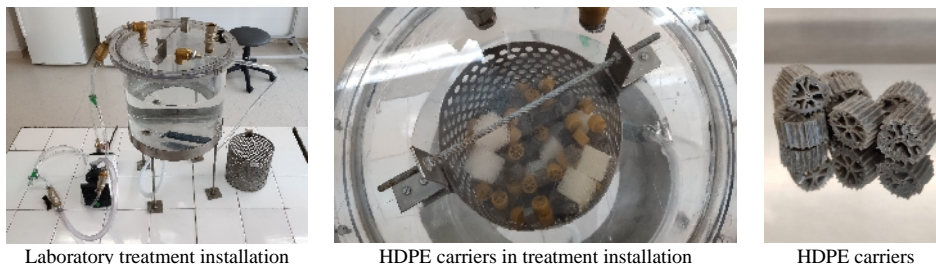
Figure 2. Bio-augmentation of HDPE structure
