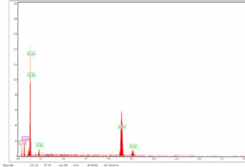
Figure 4. The EDS spectrum of the ZnO/PDMS powder, ultrasonic
