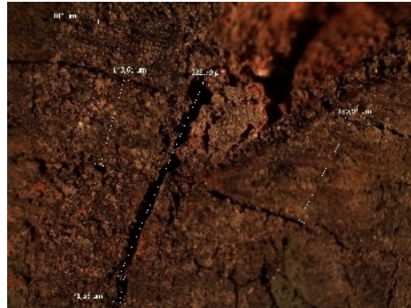
Figure 5. Crack size and orientation
