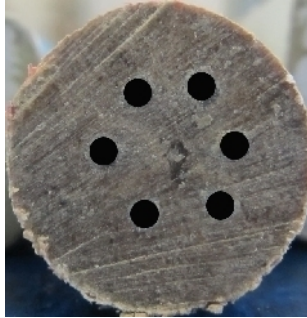
Figure 5. The position of reinforcements (black circles) into the profile
