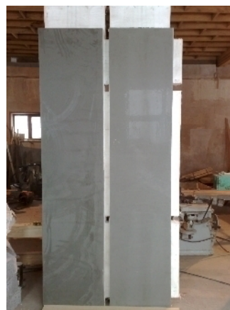
Figure 2. Prototype of the wall panels made of glass fiber reinforced mineral matrix
