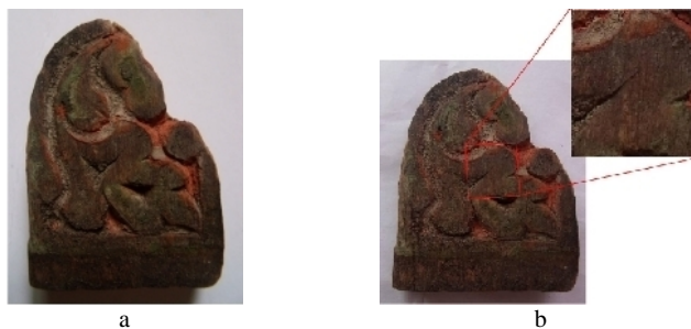
Figure 4. Sample of window frame, analyzed on stereomicroscope (a), analyzed by MicroXRF (b)
