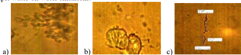
Figure 3. Optical microscopy images (1000x) of emulsions structures: a) honeycomb of HK emulsion; b) honeycomb of MC of; c) chain structure of HC emulsion
