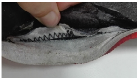
Figure 7. The aquablock overlap and stitching forming a hard point (personal archive)
