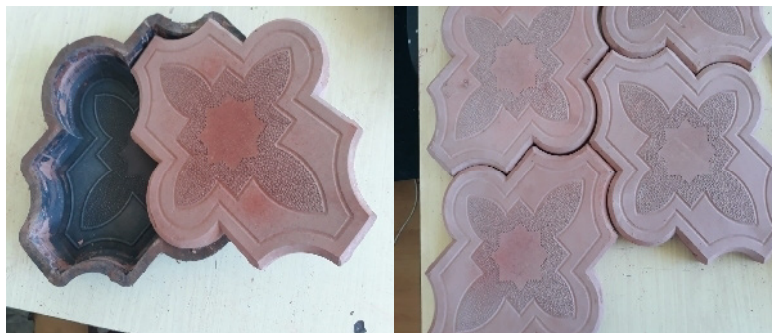
Figure 2. Paving blocks with leather fibers
