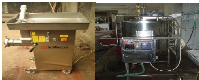
Figure 1. Hydrolysis equipment (grinder for pelt waste and autoclave)
