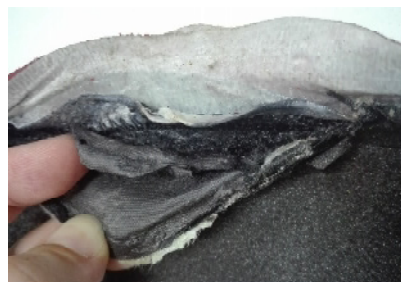
Figure 8. Two overlapped OutDry® membranes identified in the tested pair of hiking boots (personal archive)
