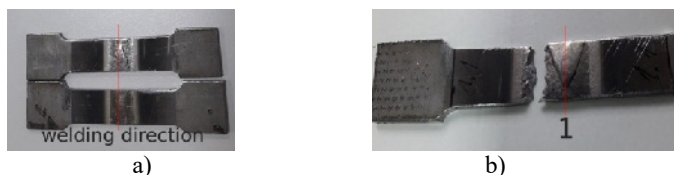
Figure 1: a) specimens for tensile testing; b) fractured specimen
