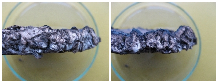
Figure 2. Biocomposite section highlighting microbial development
