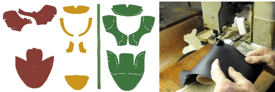
Figure 3. Upper pattern template, stitching operation
