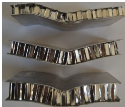
Figure 6. Damaged samples after three point bending test
