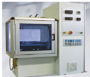
Figure 1. Electric press used to process specimens (for physical-mechanical testing)
