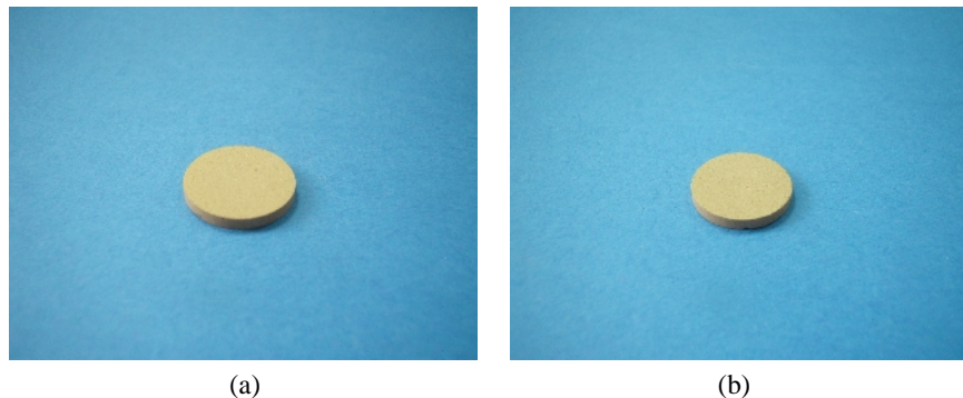
Figure 1. Photographs of specimens (diameter: 13 mm) made of ash mixtures (FA/BA:1/1) and sintered via the two-step method: (a) TSS1 and (b) TSS2
