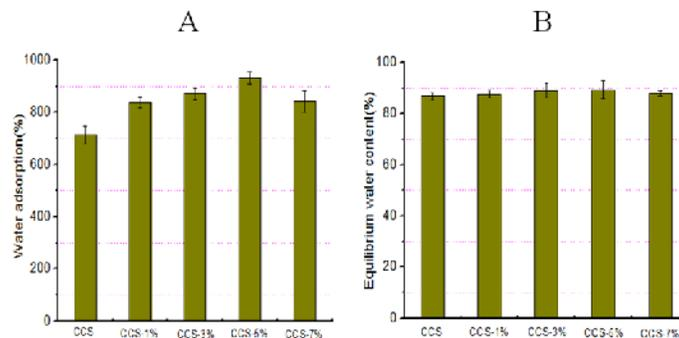
Figure 2. Water adsorption and equilibrium water content of COL-CS (CCS) scaffold containing different concentration of nano-TiO<sub>2</sub> (0,1,3,5,7%)
