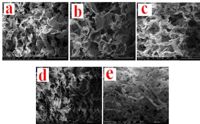
Figure 1. SEM images of cross sections of COL-CS scaffolds with various concentration of nano-TiO<sub>2</sub> (0,1,3, 5 and 7% represented as a, b, c, d, e, respectively)
