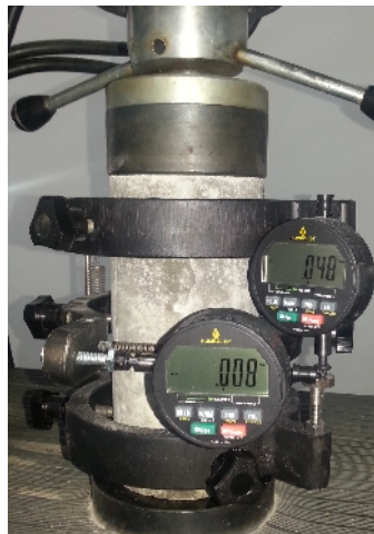
Figure 1. Measuring modulus of elasticity in compression
