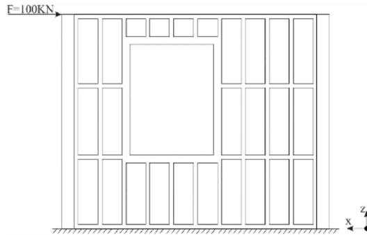
Figure 3. Loading schema of the GFRMC structural wall
