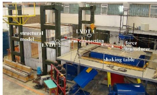
Figure 2. Structural model laterally connected to shaking table
