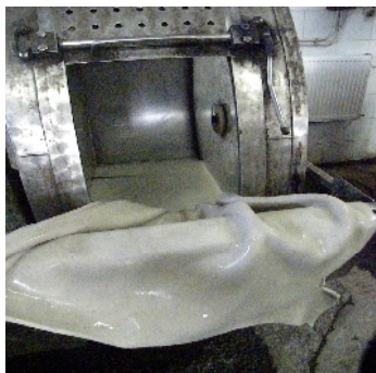
Figure 8. Tanning drum used in pre-tanning tests on pilot scale
